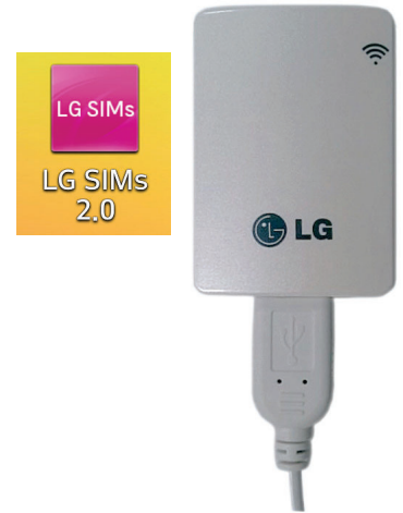
Figure 134: SIMS WLAN Module to DFS System Example.
